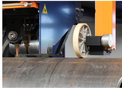
For accurate cuts, the RBPC can measure and compensate longitudinal movement of the pipe during rotation (creep) and circumference deviation of the pipe.
