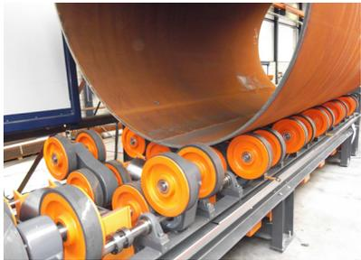
The roller bed is used to rotate and support the pipe. The tandem wheel sets can smooth unevenness of the pipe surface (like weld seams) to prevent vibrations during cutting and obtain accurate cuts.
